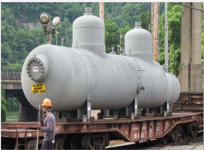
Horizontal Steam Generator
